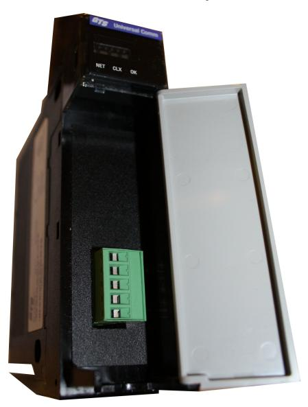
The CLX-422-IPC connects a ControlLogix controller to a Honeywell® IPC-620 Serial I/O bus.
