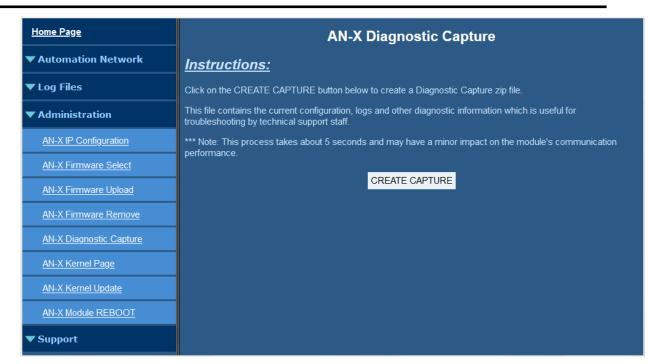
Click the CREATE CAPTURE button to create the file. There is a slight delay while AN-X builds the file.
