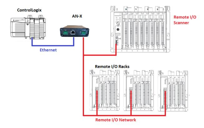
The RIO-ADPT communications module connects a ControlLogix PLC or other device to an Allen-Bradley remote I/O network.
