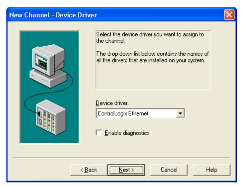
3. For the *Device Driver*, select the *ControlLogix Ethernet* driver and click *Next*
