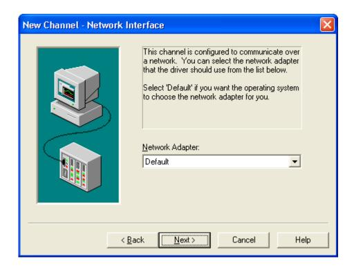
4. Select the *Network Adapter* that is connected to the AN-X-DHP. If there is only one network adapter in your computer, leave it set to *Default*. Click *Next*.
