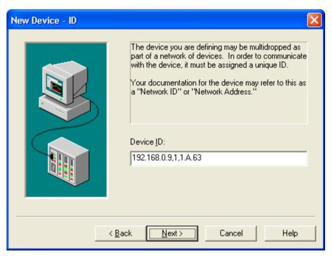
10. *Enter the Device ID*. This is the path to the destination PLC-5. The first four numbers are the IP address of the AN-X-DHP. This is followed by a comma, a 1 (to indicate the backplane, another comma, then 1.A. and finally the PLC-5 station address in decimal. The AN-X-DHP emulates a 1756-ENET module communicating through a 1756-DHRIO module in slot 1. Click *Next*.
