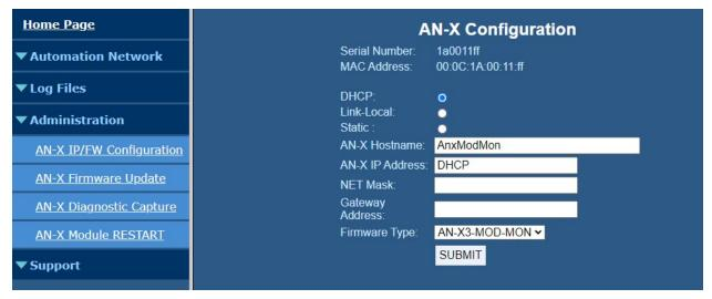
The serial number and MAC address of the AN-X being configured are shown.
