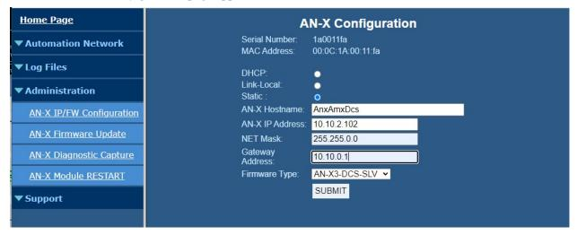
The serial number and MAC address of the AN-X being configured are shown.
