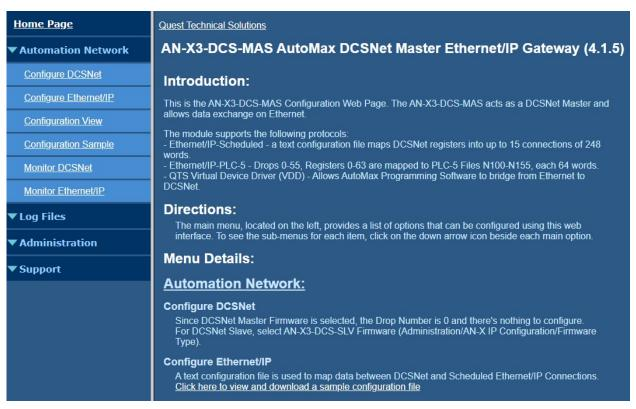
The left pane contains commands. Click on the arrows at the left of the main headings to expand or contract the sections.
