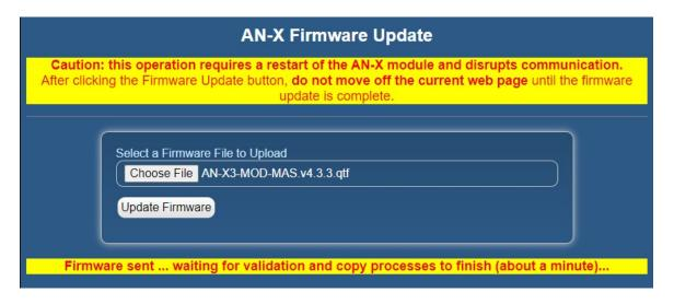
When the update is complete, AN-X displays a message that indicates the success or failure of the update.
