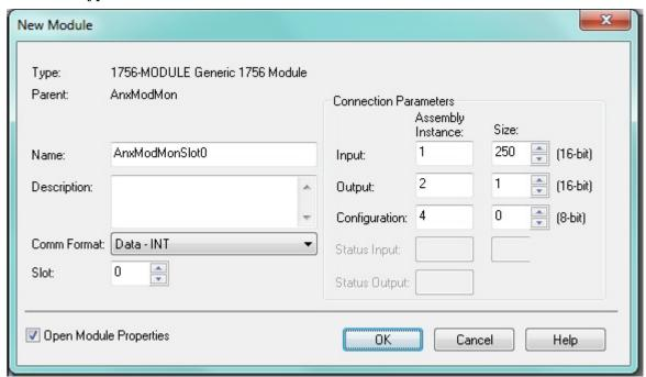
Set the parameters as shown. Even though there's no output data, we have to set the Output Size to 1 since RSLogix 5000 won't accept a size of 0.
