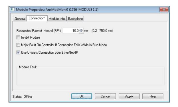
Repeat these steps for slot 15. The only differences will be that the slot number will be 15 instead of 0 and the RPI can be much longer (for example, 500 ms) for the diagnostic connection.
