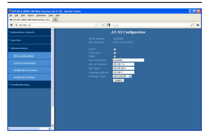
The top of the screen shows the serial number and MAC Address of the AN-X2 being configured.
