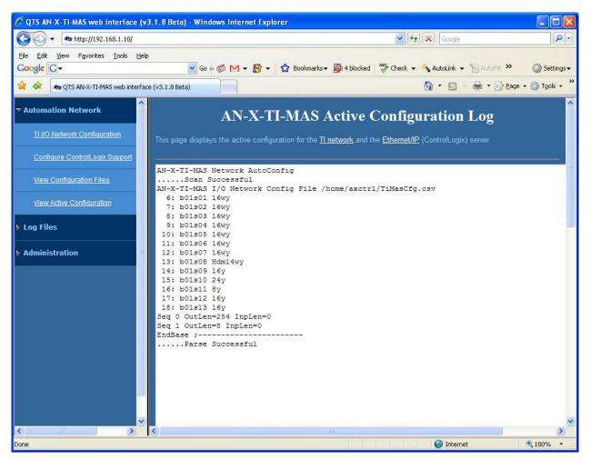
Click the *TI network* link to view the current I/O network configuration.
