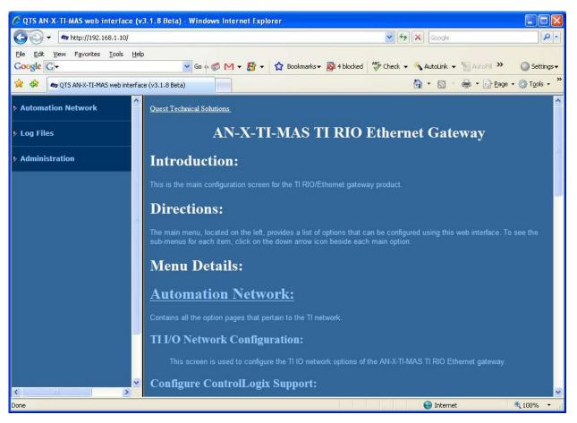
The left pane contains commands. Click on the arrows at the left of the main headings to expand or contract the sections.
