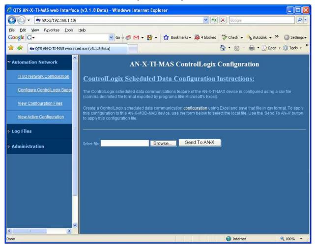
Type or browse the configuration file name into the *Select file:* area. Then click the *Send To AN-X* button to send the file to AN-X.
