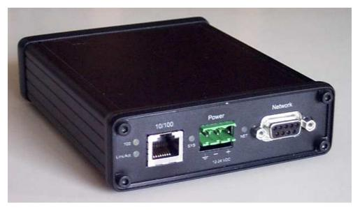
The AN-X-TI-MAS communications module connects a ControlLogix PLC or other device to a TI 505 remote I/O network.
