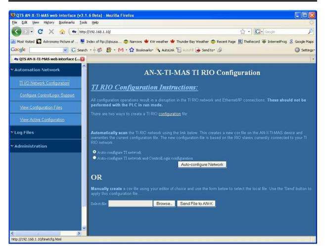
AN-X can generate a default ControlLogix data mapping configuration based on the I/O it finds (see page 24). If you want AN-X to generate the ControlLogix configuration, check *Auto-configure TI network and ControlLogix configuration*. Otherwise, check *Auto-configure TI network* (the default).
