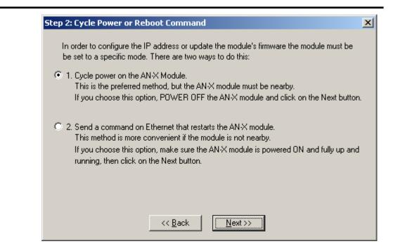
The preferred method is to cycle power on the AN-X. Select the first option on the screen and click the Next >> button.
